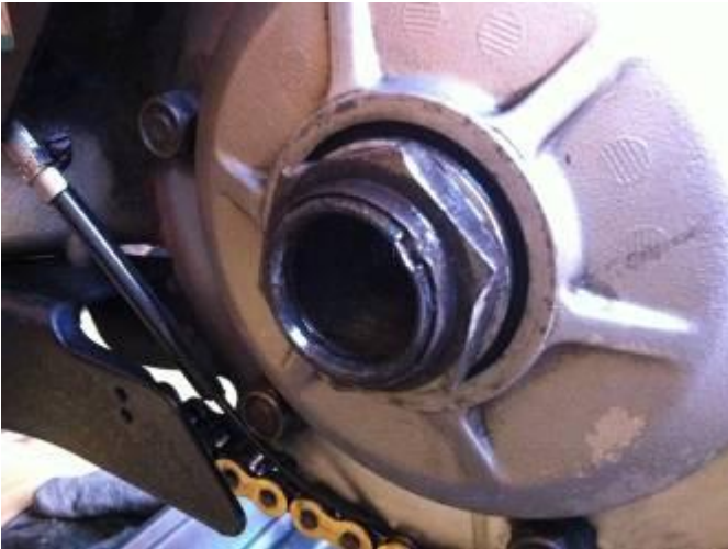
Figure 2: Axle Nut Unstaked
