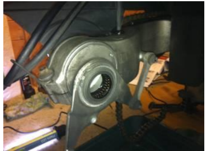
Figure 8: Axle Removed, Check Bearing and Clean Area
