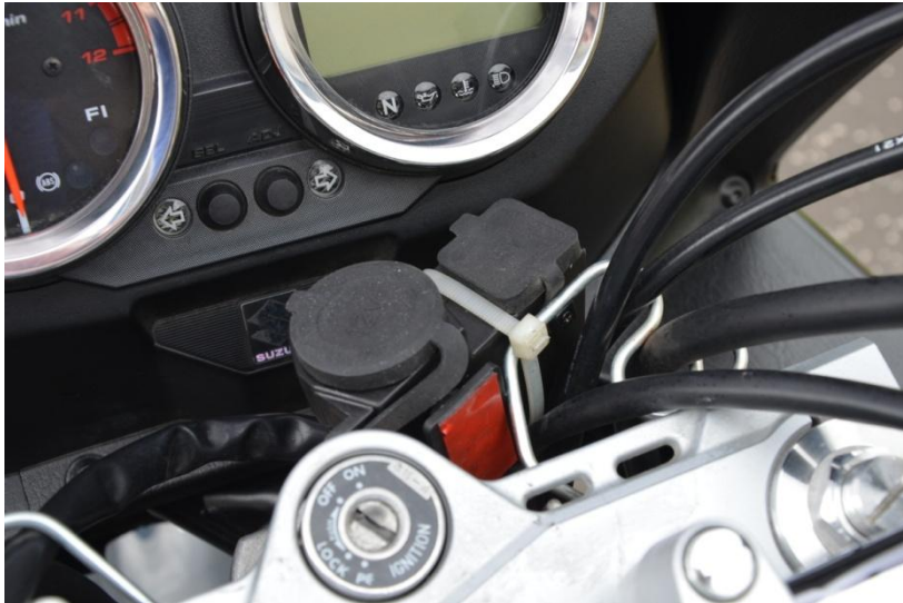
Power unit mounted to steering yoke
