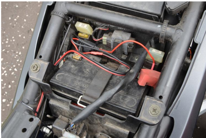
Wires connected to battery, inline fuse just behind it
