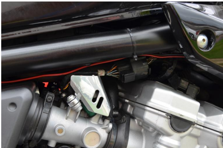
Red/black wires tied to frame rail
