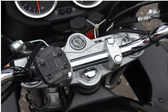
Handlebar mounting for phone
